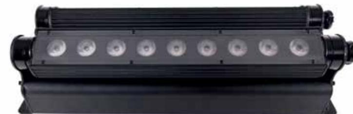
The CLF LEDwash XL is a unique, one-of-a-kind wash fixture with two LED segments. The two horizontal LED battens can be manually tilted and controlled separately. Because of the 30° and 50° lens it is possible to use the fixture as wallwash with both parts complementing each other. Besides that, the fixture can be used to illuminate two different surfaces simultaneously.
